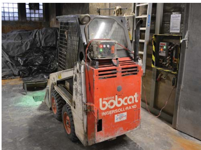
A compact wheel loader conveys the material for the extrusion press through the material drop into the extruder.
